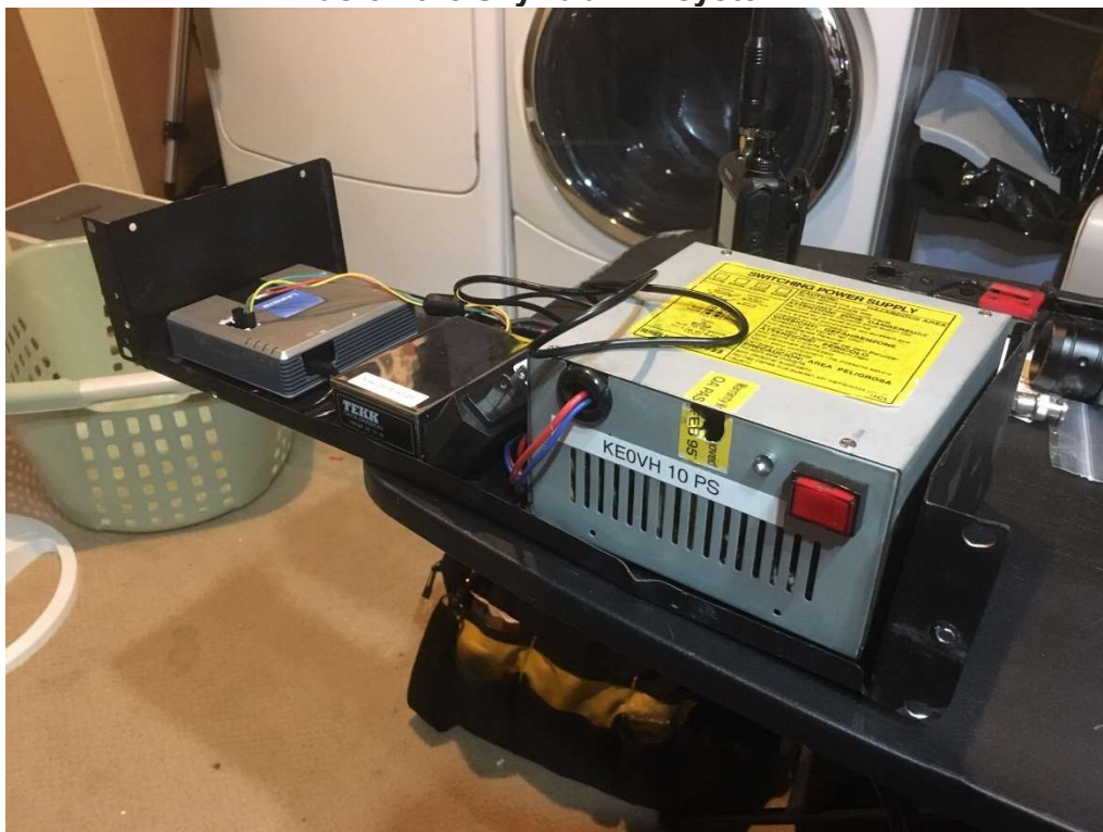
MORE PROJECTS. The KE0VH Office node utilizing an empty Linksys box as a case for a Raspberry Pi3 and MMDVM modem board running the Pi-Star software. The shiny box in the middle is a small Tekk data radio on 442.700 Mhz. So if you talk to me while I am in Lakewood, this is the setup being used to link into the SkyHubLink system.
