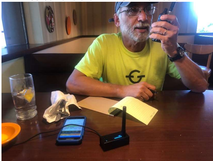
The equipment setup in the restaurant. You can see the SKYHUB AllMon display on the cell phone screen and the NETCONTROL below
