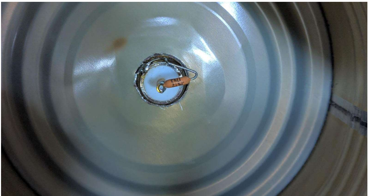
The resistor (sensor) inside the can
