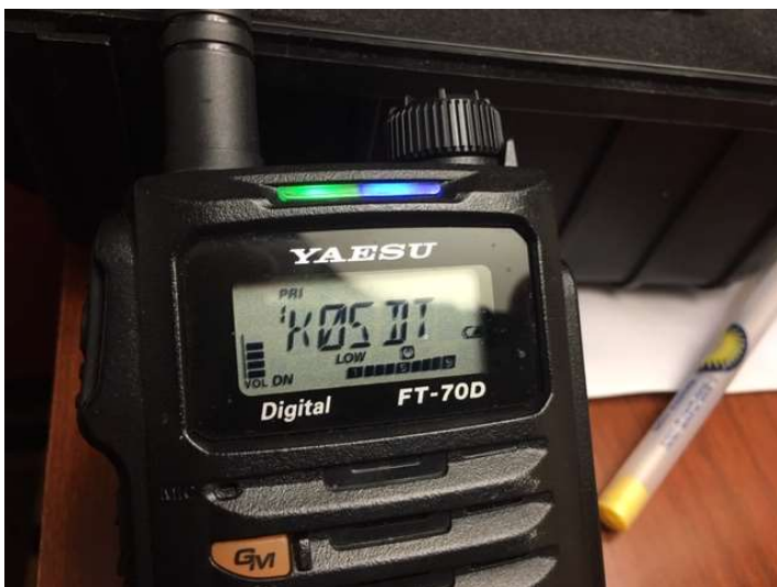
Talking to Shane KØSDT in Montana while in the hotel room in southern Colorado via Yaesu Fusion mode to DMR with the Zumspot hotspot
