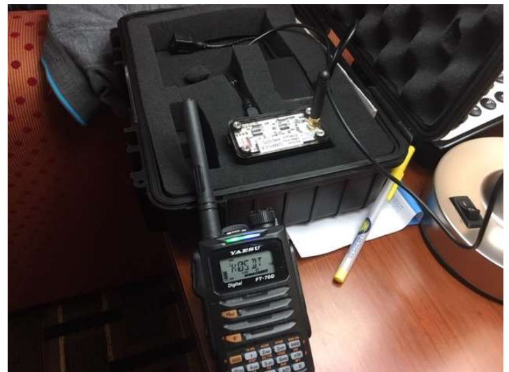
Talking to Shane KØSDT in Montana while in the hotel room in southern Colorado via Yaesu Fusion mode to DMR with the Zumspot hotspot
