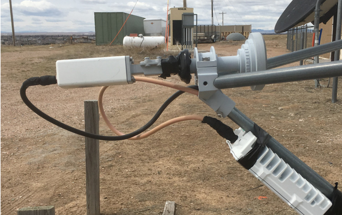
The BUC just temporarily taped up until the new mount arrived
