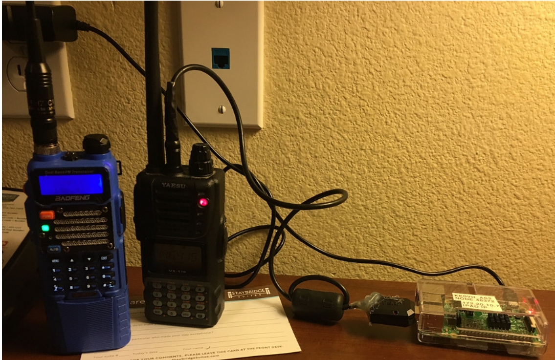
The Baofeng UV-5R handheld that is my general carry around HT, and the portable AllStar Raspberry Pi3 and Yaesu FT-170 that is my 2 meter “node” radio.
