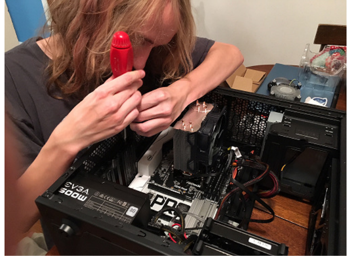
Installing a new mother board, processor and cooling tower in the Chassis
