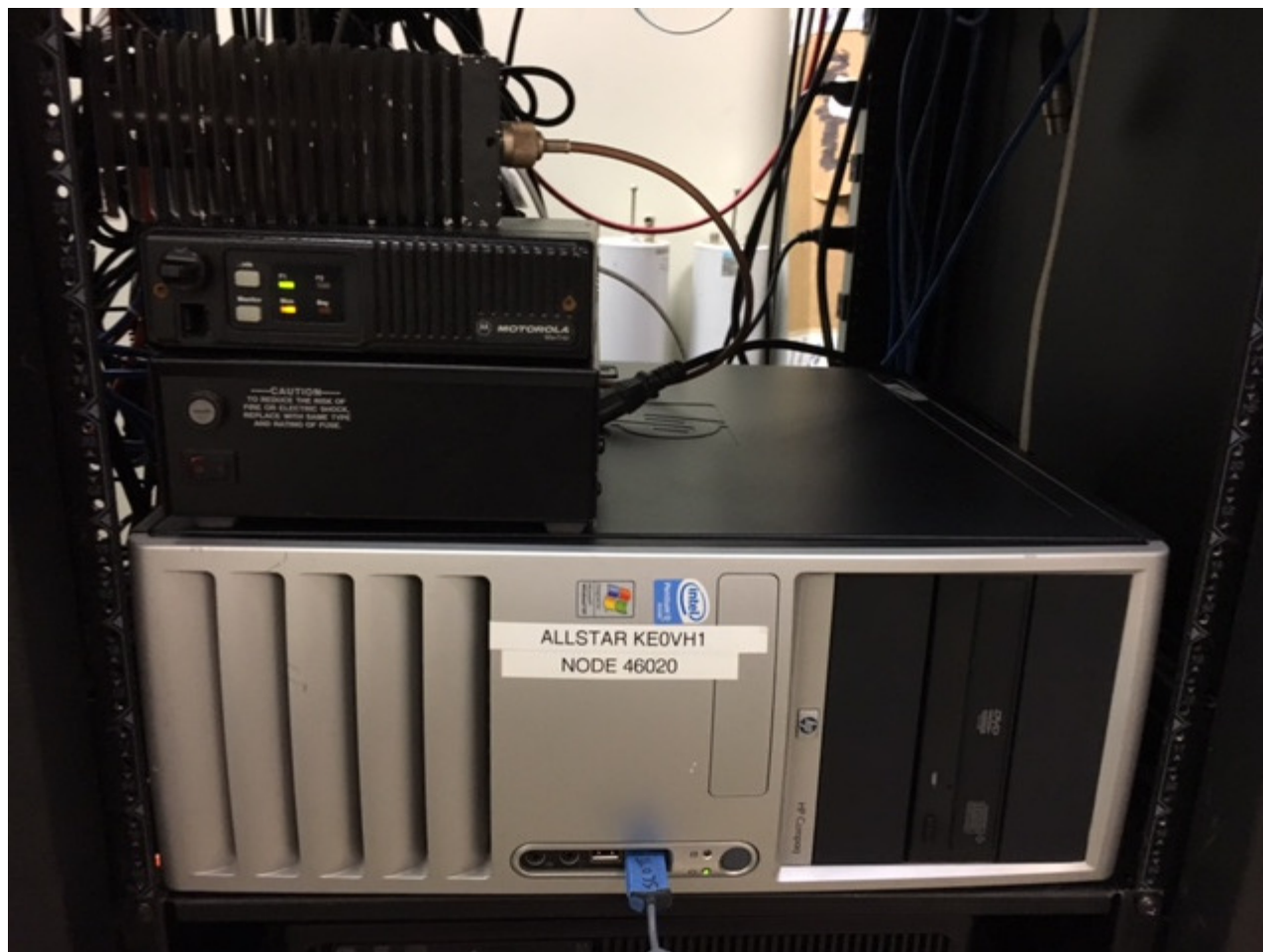
The KE0VH AllStar node in the rack operating with a re-frequencied re-purposed Motorola Maxtrax radio as the simplex repeater radio.
