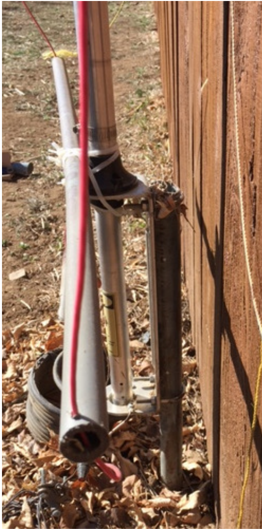
Side view of the original mount and the wind broken spar and “spider”
