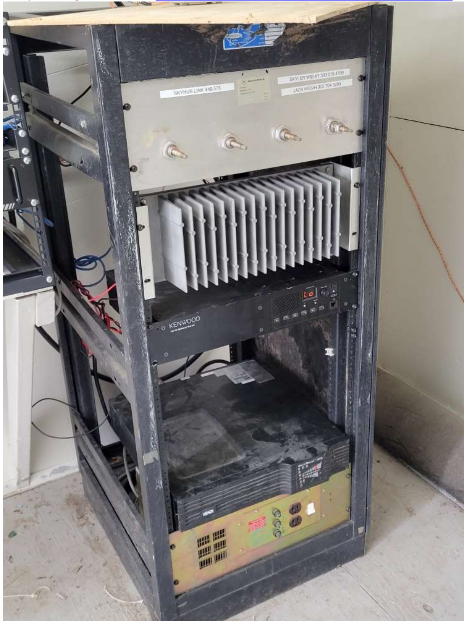
The SkyHubLink Bakulite Mesa 449.575 analog AllStar repeater, with space for the NEW Wires-X repeater in the rack.
